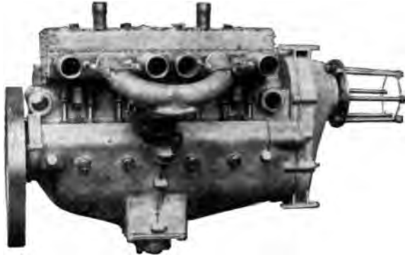
Fig. 30. Four-Cylinder Type with Gear Drive to Propeller Shaft
